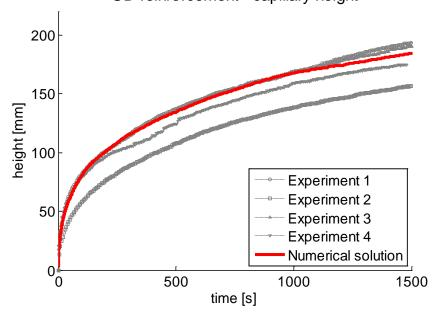
UD reinforcement - capillary height
