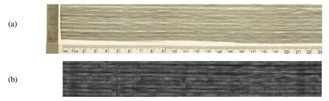
**Figure 1:** Image (a) is an original picture of the fibrous reinforcement. Image (b) shows the grey level mapping obtained after processing in order to evaluate the local fiber volume content.
